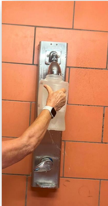
City staff measuring flow rate of shower at Salt Lake City Sports Complex.
