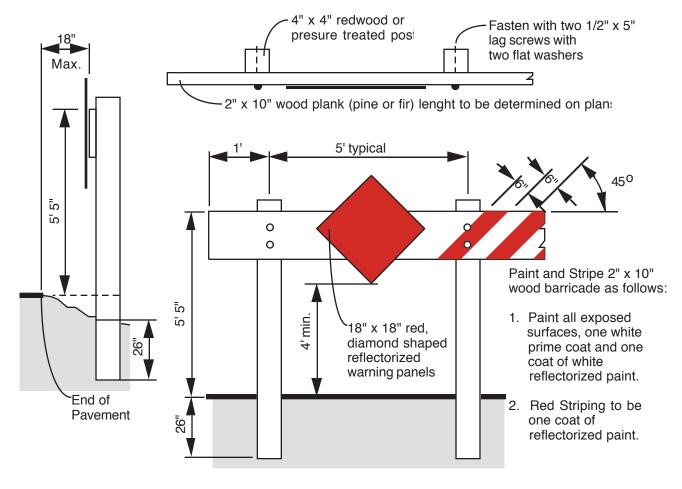
The Barricade must extend to the pavement edge if there is a roll curb or no curb. The Barricade must not be further than 4 feet from the fence of a vertical curb.
