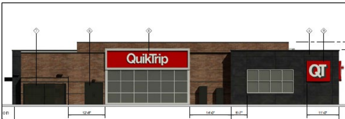
North elevation facing 400 S, façade features non-transparent glazing and signage
