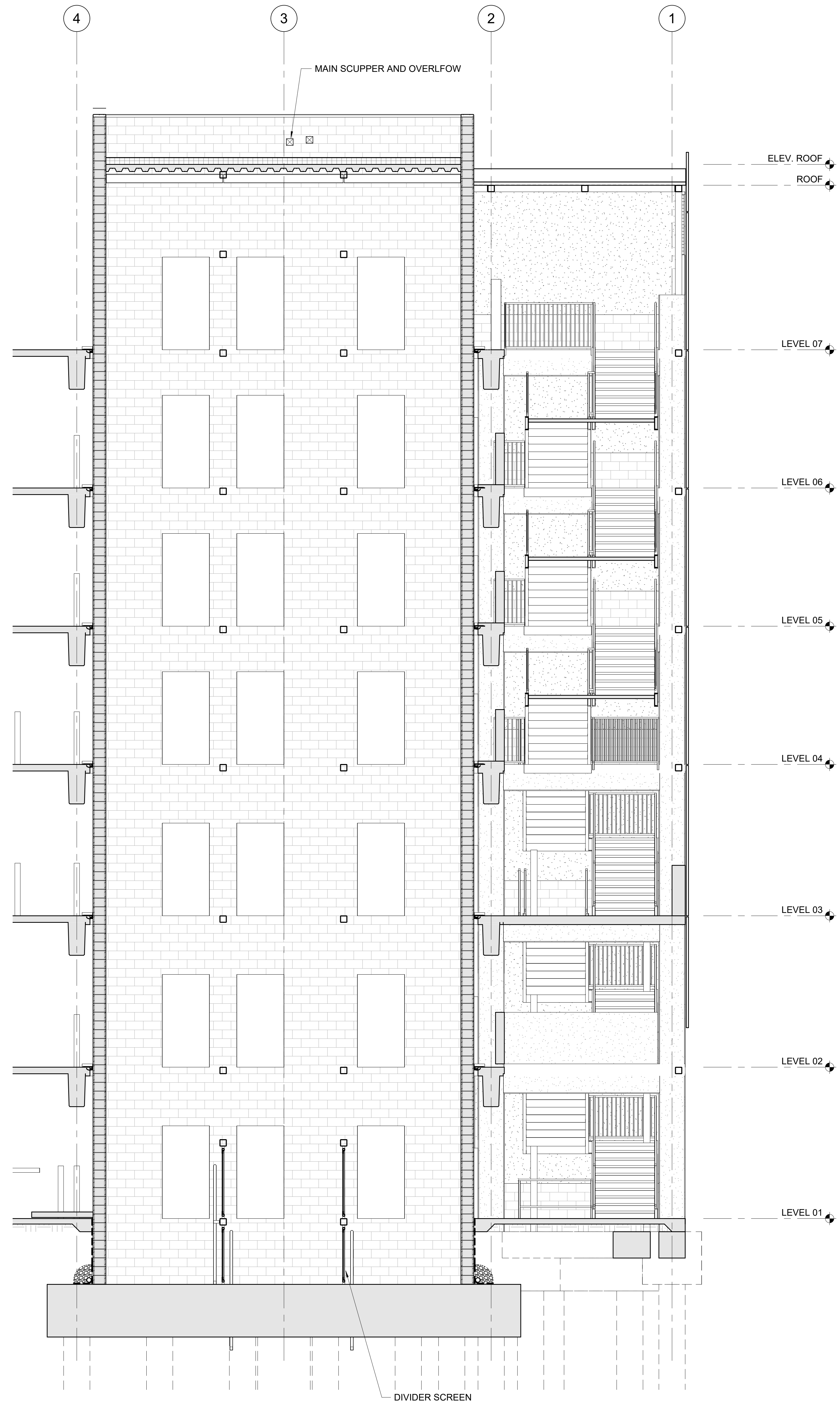
1 ELEVATOR & STAIR CORE #1 ENLARGED SECTION 1/4" = 1'-0"
