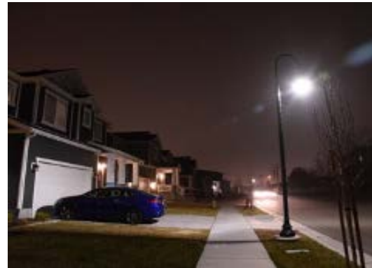
A pedestrian light with inappropriate light distribution and poor shielding creates a significant amount of light trespass on a nearby residence.
