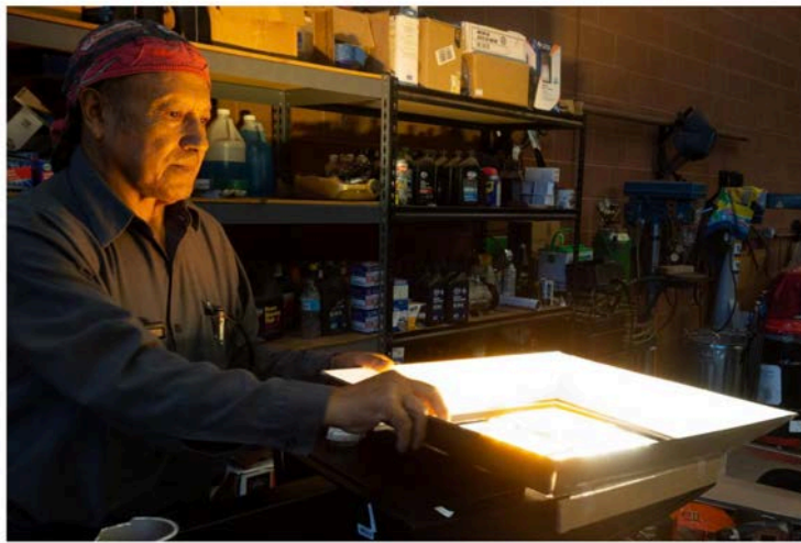
Ivins Fleet Mechanic Wilson Jimenez fits a shield onto his light-filter prototyping station in the city garage. He designed the amber insert that adapts the city's LED bulbs to be "night sky friendly" and has custom-built about 150 inserts to date. CREDIT DAVID FUCHS / KUER
