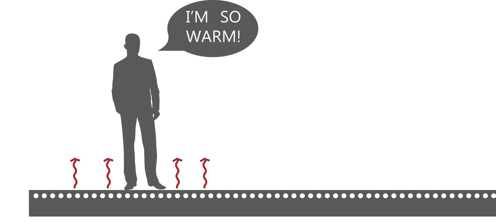
**Cooling:** LOOK UP and see the high volume, low velocity fans that cool the apparatus bays. **Air movement improves your body's natural cooling mechanisms**, keeping you happy, safe and productive. High volume, low velocity fans also use a fraction of the amount of energy that a traditional A/C system would require.
