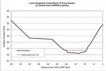
Figure 5. Surveyed stream channel cross section plots illustrating the variability in channel shape within the WHOS property.
