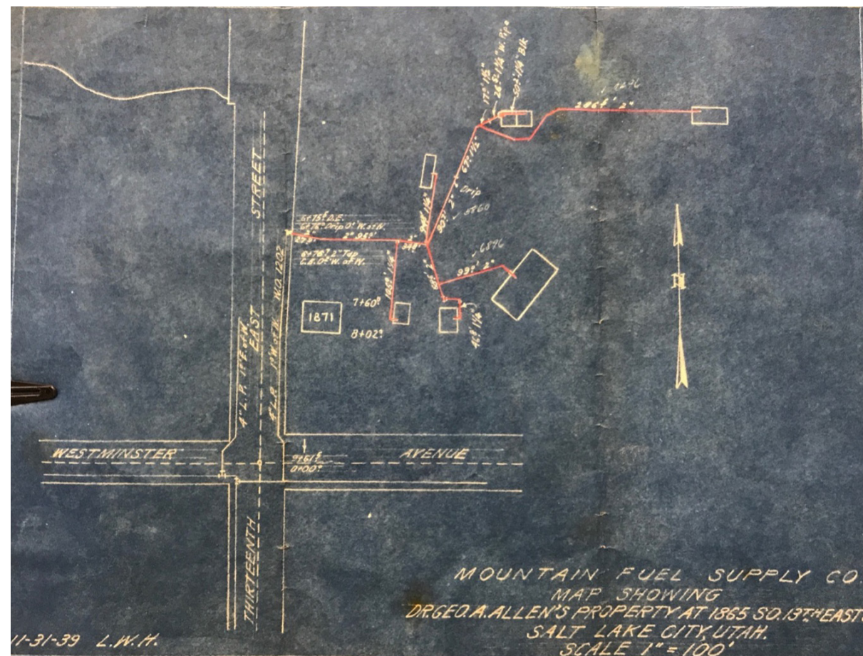
Figure 2-23. The six buildings that compose lower Allen Park Drive were connected to natural gas lines by Mountain Fuel Supply Co. in 1939. (M-2-H)
