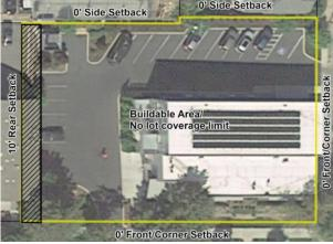
Buildable area if the property is rezoned to CB. There would be no lot coverage limit, except for the rear (west) setback. Building additions over the size threshold would trigger Design Review and additional design guidelines.
