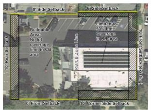
Buildable area with current split-zoning. A ~950 square foot addition could be built on the east half of the property under the current zoning by right. An addition without such size limitations could be built on the west side.
