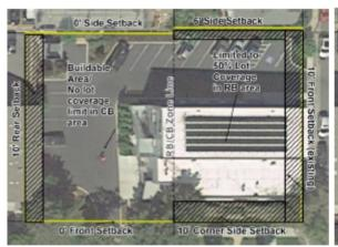
Buildable area with current split-zoning. A  $\sim$ 950 square foot addition could be built on the east half of the property under the current zoning by right. An addition without such size limitations could be built on the west side.
