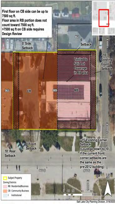
This graphic illustrates potential footprint options based on the RB zoning requirements (provided by the SLC Planning Division). The existing front setback would allow for just under 5' of growth to the south (900 South). Within the confines of the 50% lot coverage there is room for growth to the north along 1000 East. As these aerials illustrate, that area is currently in use as and provides 5 standard and 1 ADA stall of off-street parking (at 45 degrees).
