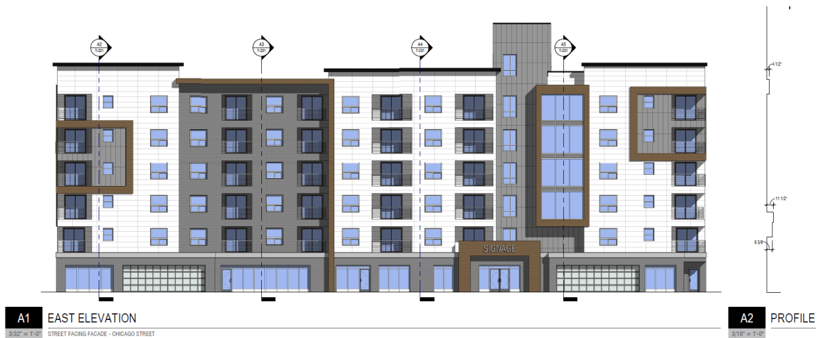
Figure 3 Example of the impact to the building design reducing the vertical clearance requirement to 9' has on the same 45 N Chicago St project. The loading area can be located inside the parking garage reducing the driveway width and freeing up space for an additional dwelling unit where the loading area used to be.
