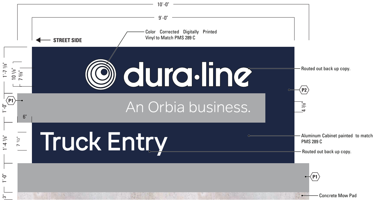
1 SIGN 05 - D/F INTERIOR ILLUMINATED MONUMENT SCALE: 3/4" = 1'-0" [1:16]
