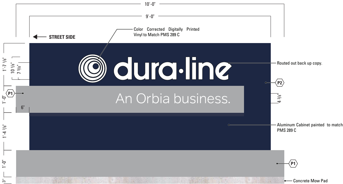
1 SIGN 04 - D/F INTERIOR ILLUMINATED MONUMENT SCALE: 3/4" = 1'-0" [1:16]
