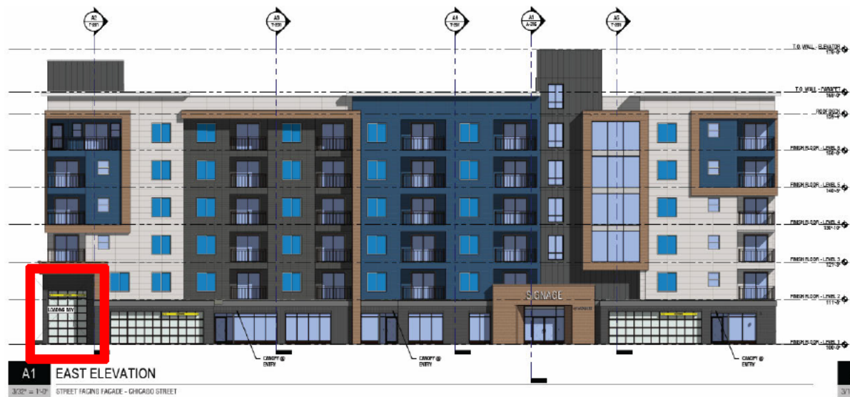
Figure 3 Full elevation of the 45 N Chicago St project showing the overall impact to the building design the required loading area creates
