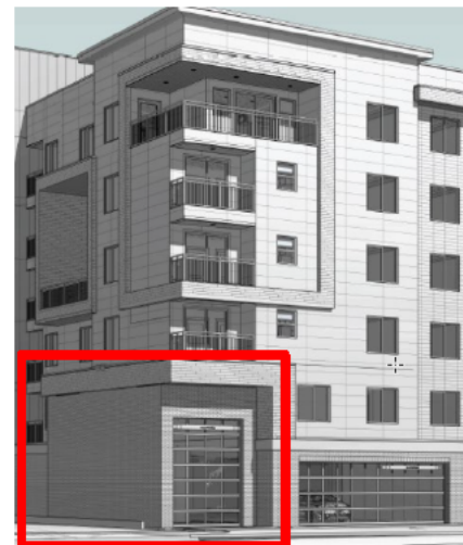
Figure 2 Example of a multi-family project at 45 N Chicago St where the loading area requirement uses space that could otherwise accommodate an additional dwelling unit.
