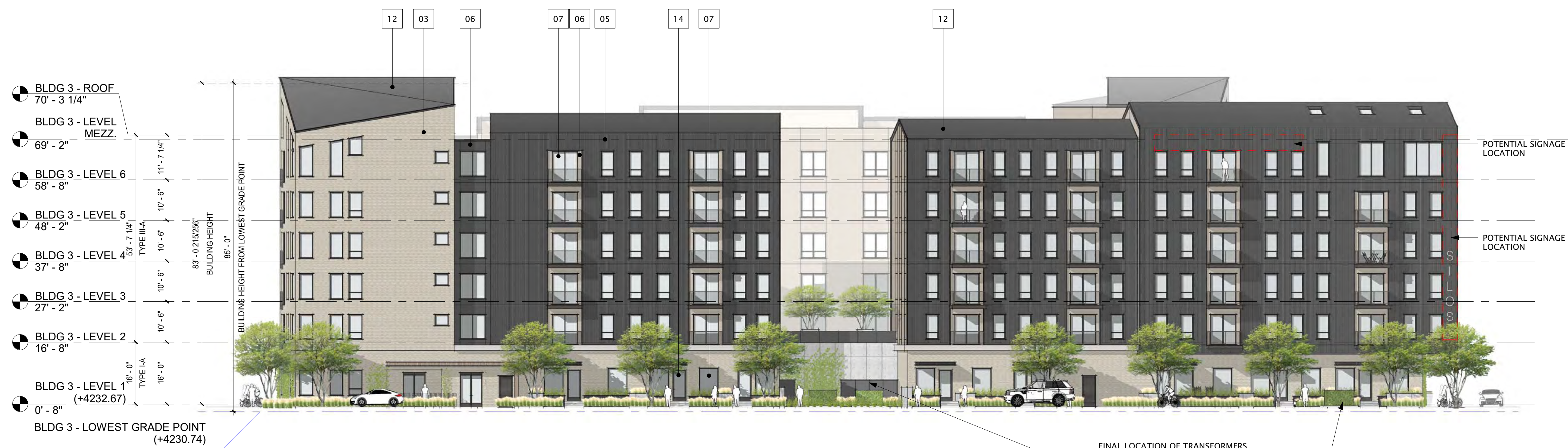
BUILDING 3 - EAST ELEVATION 1/16" = 1' - 0" 2
