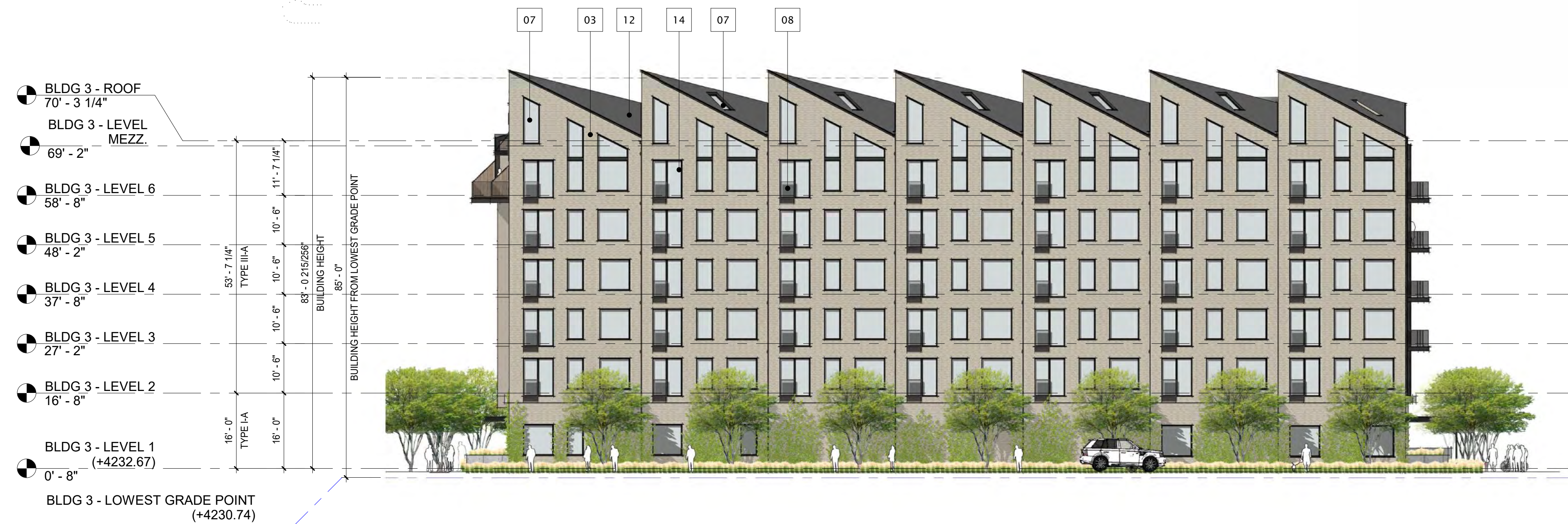
BUILDING 3 - SOUTH ELEVATION 1/16" = 1' - 0" 1
