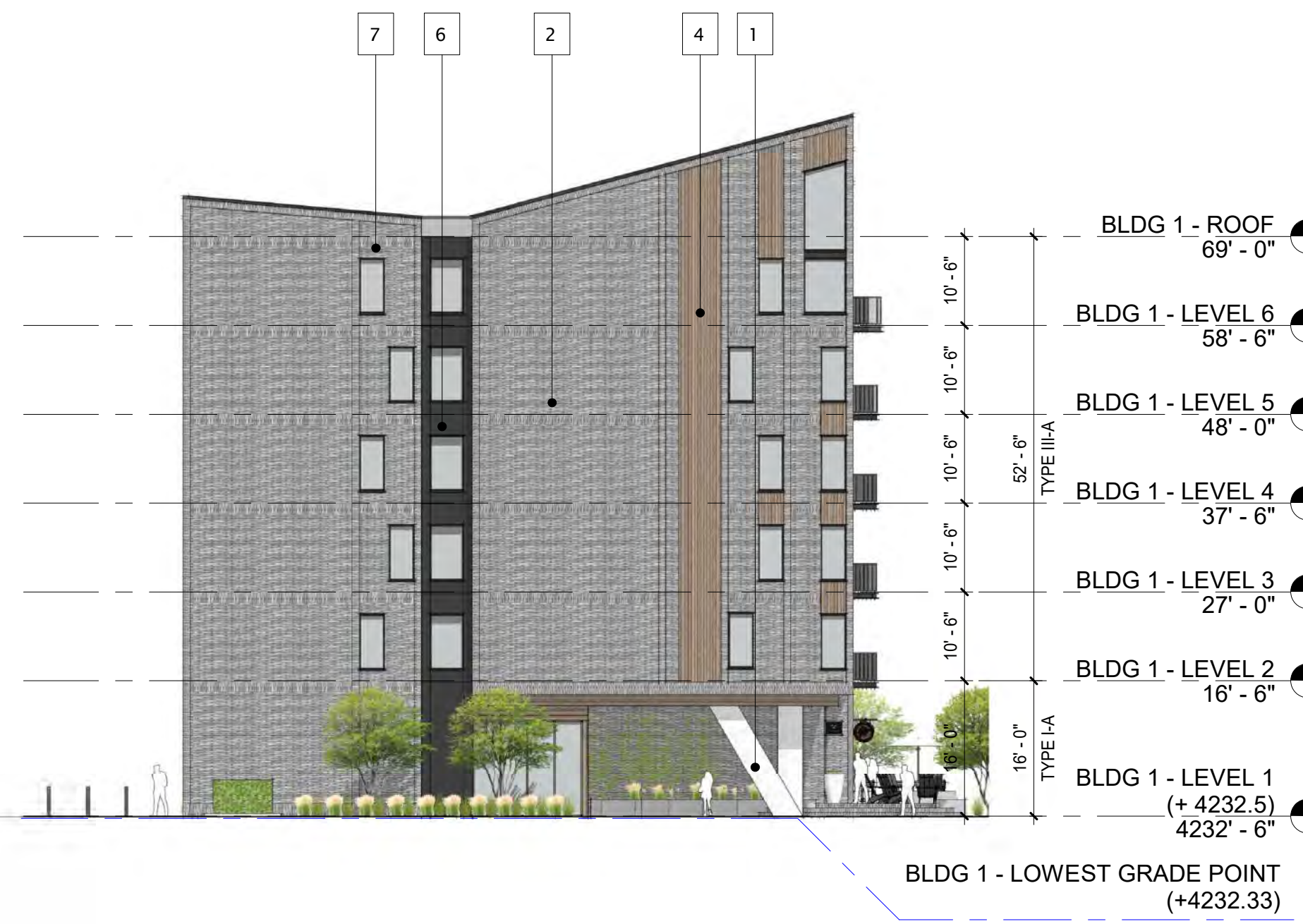
BUILDING 1 - SOUTH ELEVATION 1/16" = 1'-0" 3
