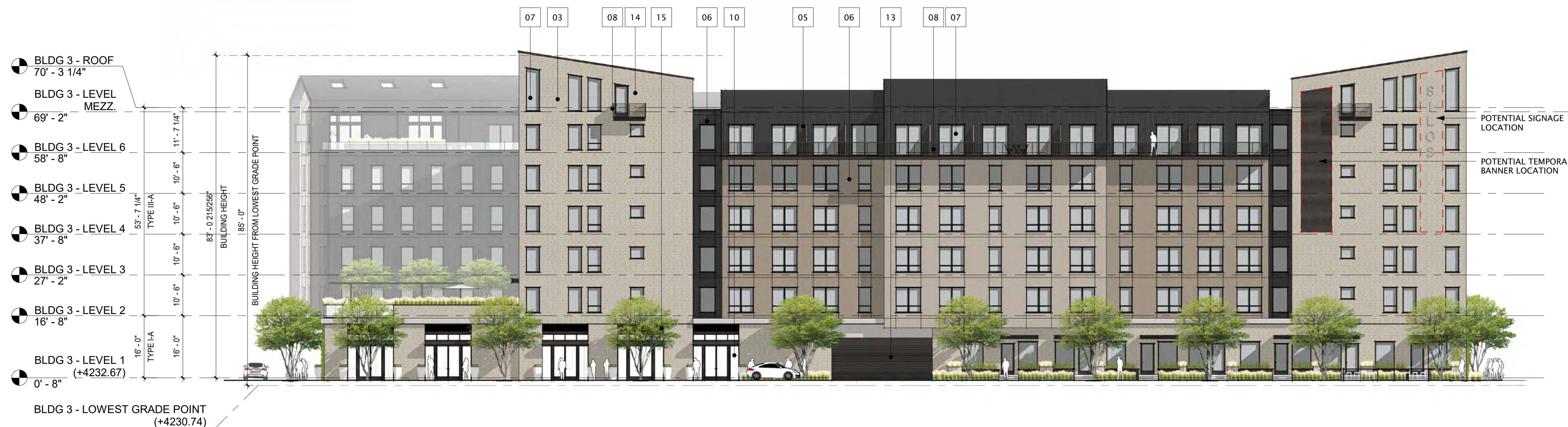
BUILDING 3 - WEST ELEVATION 1/16" = 1'-0" 2
