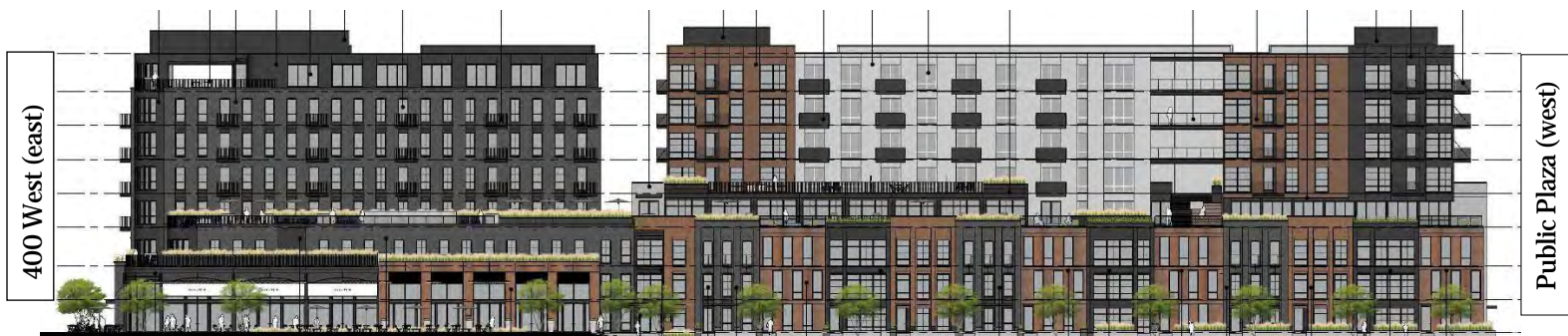
Building 2: Northern building elevation with frontage on Montague Ave (417 feet in length)
