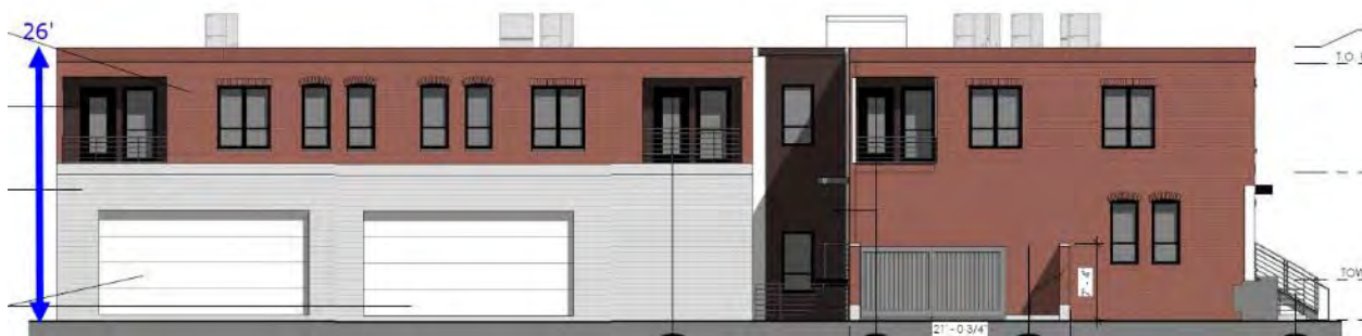
East Elevation – Building height from grade to the top of the parapet is 26'.
