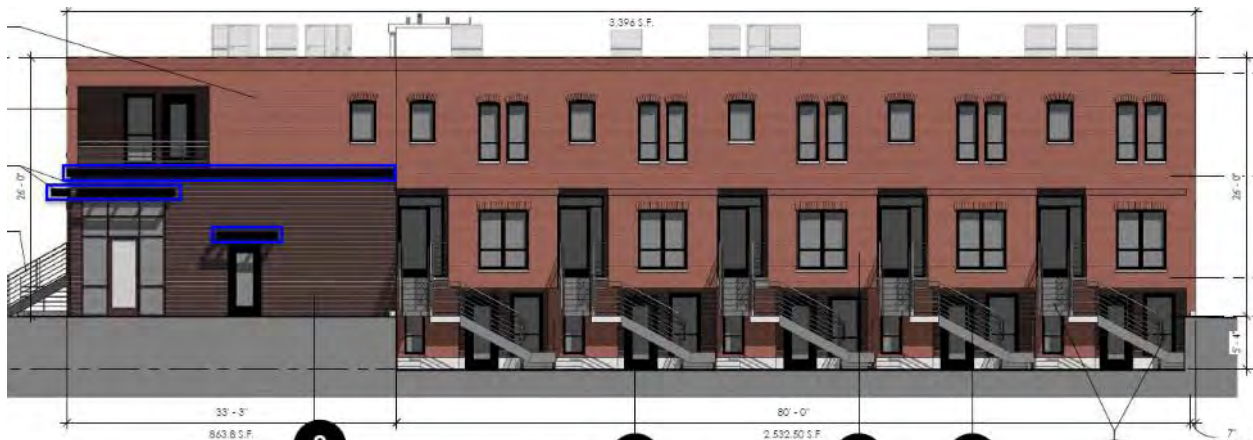
South Elevation – The canopies that extend into the setback are outlined in blue.
