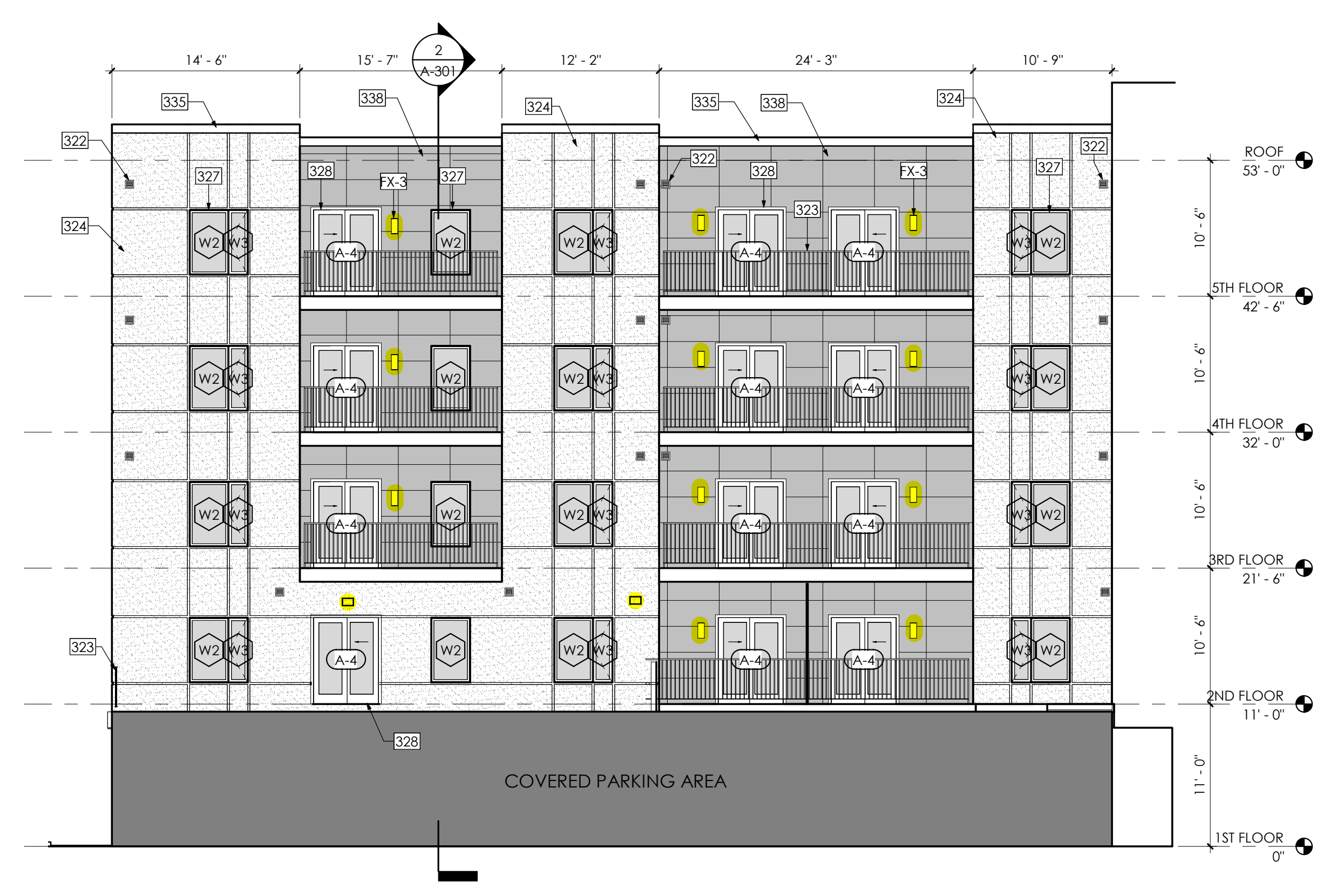
1 West Elevation Inner RAISED COURTYARD 1/8" = 1'-0"
