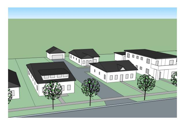
**Preservation of Existing Structure:** Center lot depicts an existing single-family home with a basement ADU, two surface parking spaces, detached two-car garage, and new, detached single-family home to the rear. This is on a larger nearly 12,000 sq. ft. lot. The three structures have a total building coverage of 27%.
