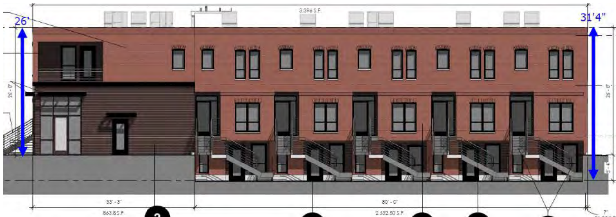
South Elevation – Additional building height requested with the Planned Development for the sunken garden level patios. The average building height from grade on this elevation is 29.8'
