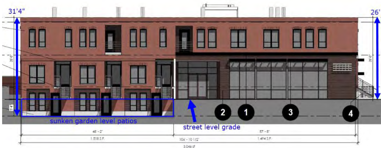
West Elevation – Additional building height requested with the Planned Development for the sunken garden level patios. The average building height from grade on this elevation is 28.5'.
