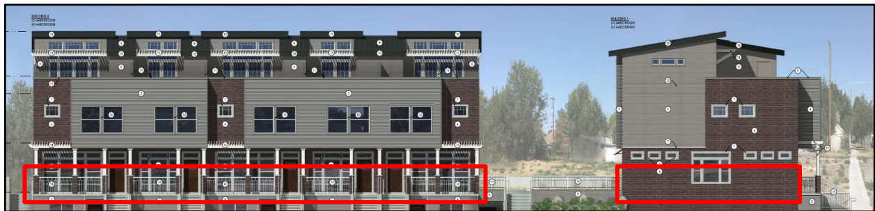
200 South and 1000 West (south façade) elevations showing the ground floor glass between 3-8 feet
