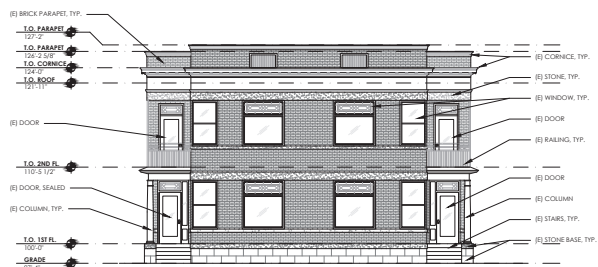
BUILDING A ELEVATION FRONT (SOUTH) SCALE: 1/8"=1'-0"
