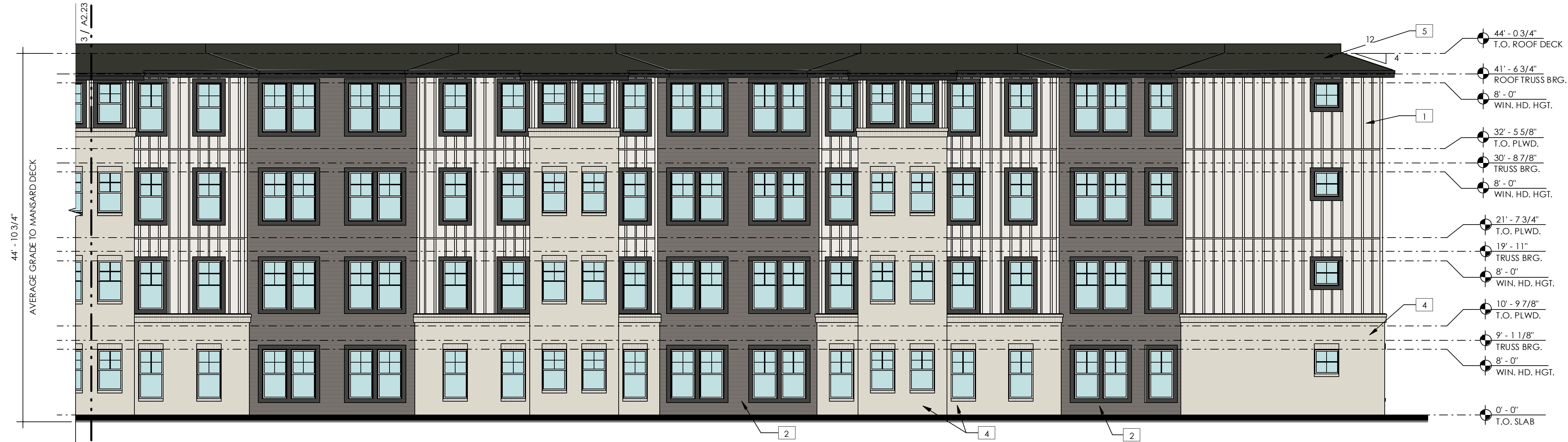
2 BUILDING TYPE II - PARTIAL SOUTH ELEVATION A
