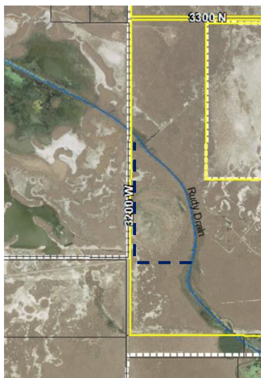
The Rudy Drain (shown in blue) crosses diagonally through the property. The developer has proposed to relocate it to the purple dashed line (approximate). The alignment is not being approved by this subdivision plat.
