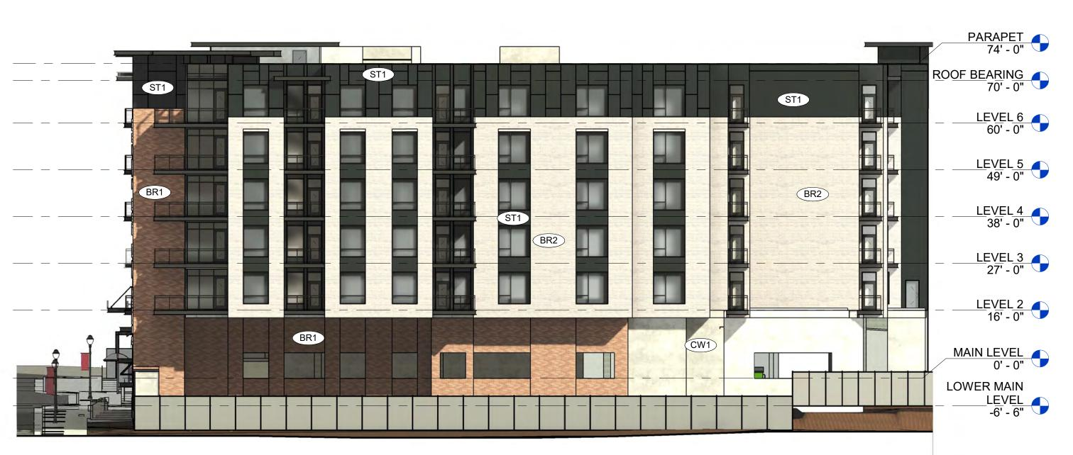
PARAPET 74' - 0" ROOF BEARING \_LEVEL 6 🔼 LEVEL 5 49' - 0" \_LEVEL 4 LEVEL 3 27' - 0" LEVEL 2 16' - 0" MAIN LEVEL 0' - 0"
