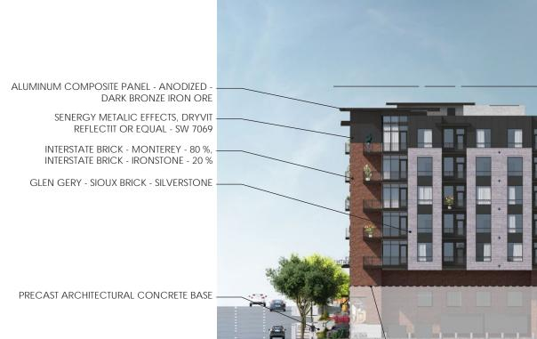
MAX BLDG. HT. 86' - 3 1/2" T.O. ROOF 79' - 0" T.O. ROOF 74' - 0"
