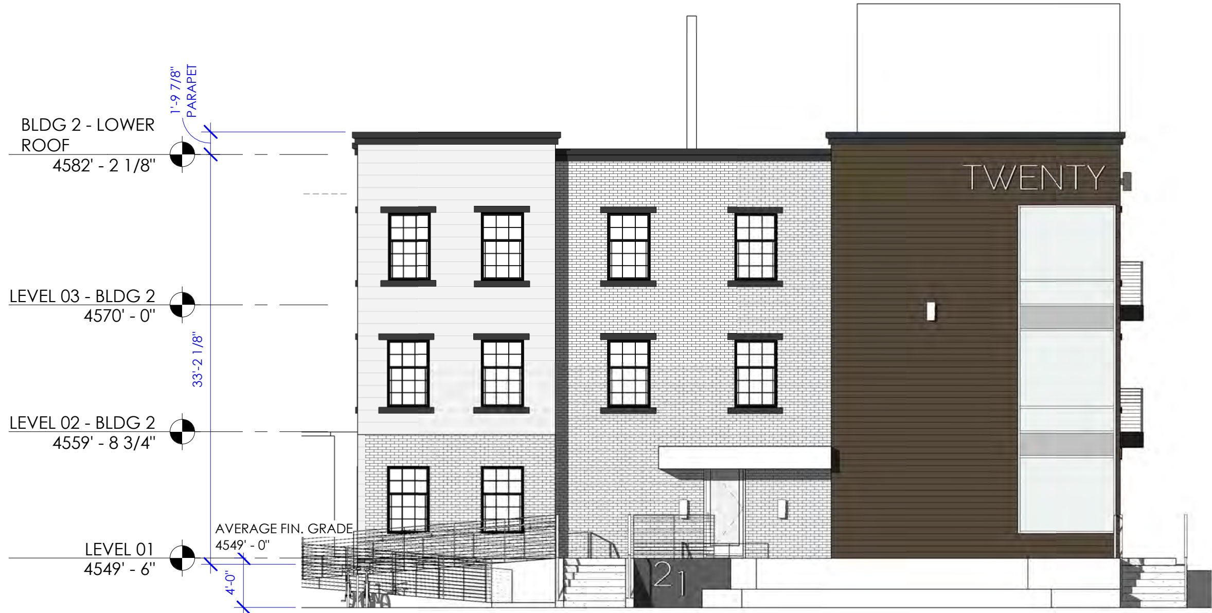
3 A206 BUILDING 2 - WEST ELEVATION 1/8" = 1'-0"
