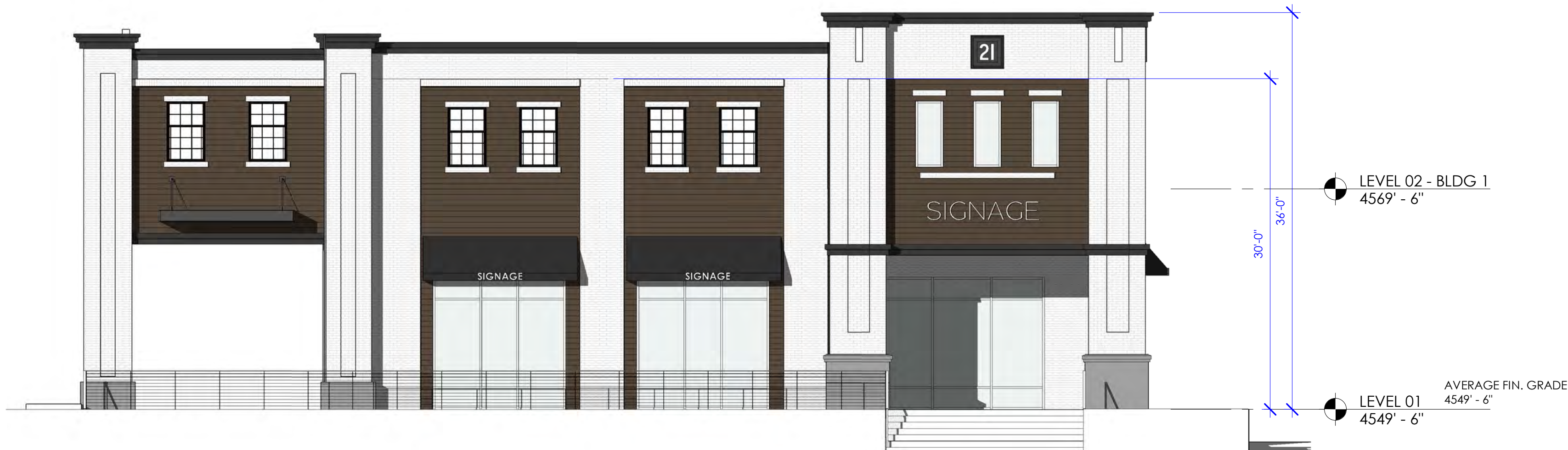
BUILDING 1 - WEST ELEVATION 2 A203 1/8" = 1'-0"
