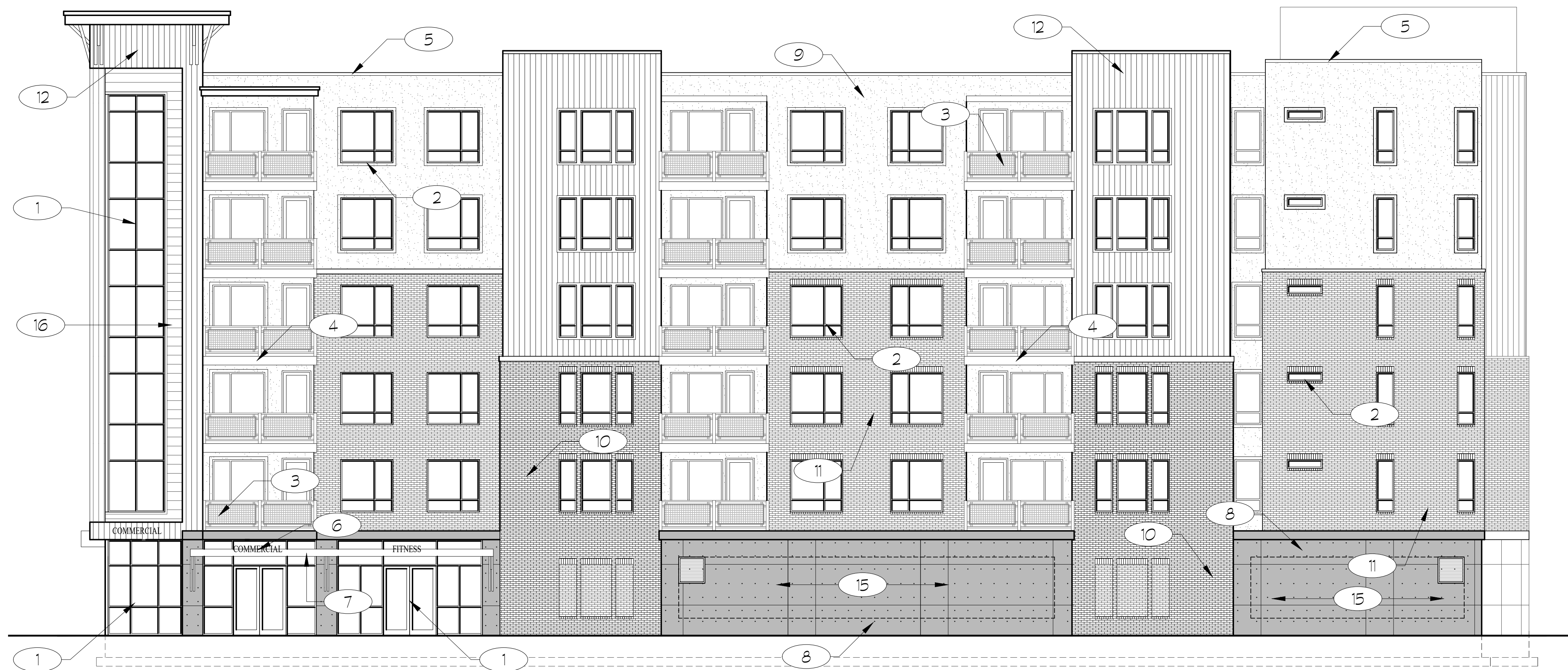
2 BUILDING ELEVATION WEST A2.02 SCALE: 1/8" = 1'-0" (24' x 36') 72% DURABLE MATERIALS
