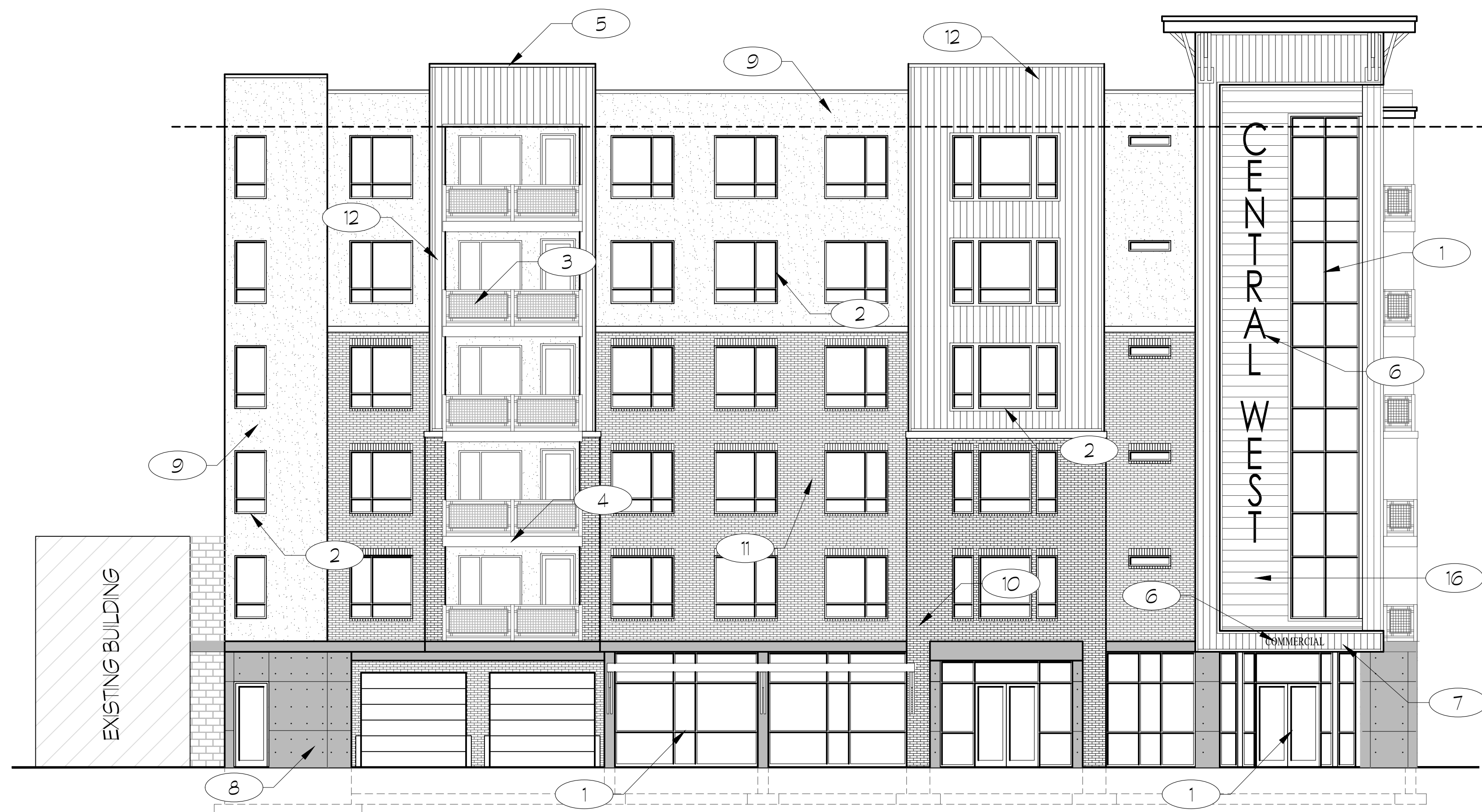
1 BUILDING ELEVATION NORTH A2.02 SCALE: 1/8" = 1'-0" (24' x 36') 73% DURABLE MATERIALS
