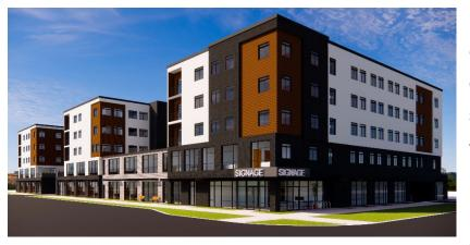
The main level is designed to engage the street frontage with a combination of building amenity spaces and residential units. The main floor has an increased floor-to-floor height (14' - 0") and with it running parallel to two main streets, it creates an ideal space and opportunity for
