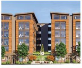
It could also be done by carrying the design of some ground level windows vertically into the upper floors. Materials and colors could be more prominent on sections of the building from bottom to top to help create the feeling of more than one building. There should be more design continuity between lower and upper floors. See example below of how long facades are broken up visually.
