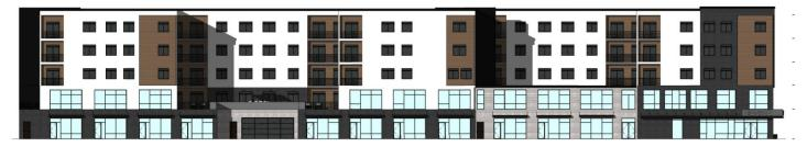
The graphics below show the area where proposed entrances exceed the allowed 40' separation. The lobby area does show additional glass between the entrances, but it is not shown as an operable door on the plans received.
