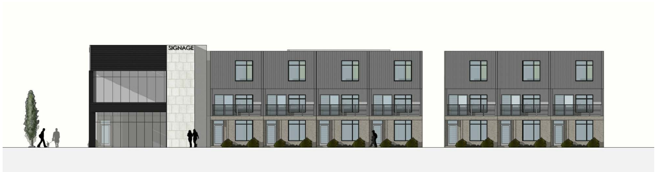
WEST ELEVATION COMMERCIAL TRANSPARENCY RATIO: 257/344sf= 74.7%
