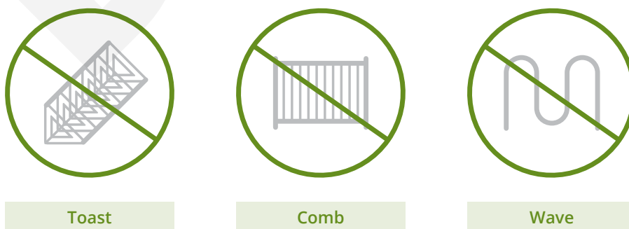
FIGURE 12 UNPERMITTED BICYCLE RACKS
