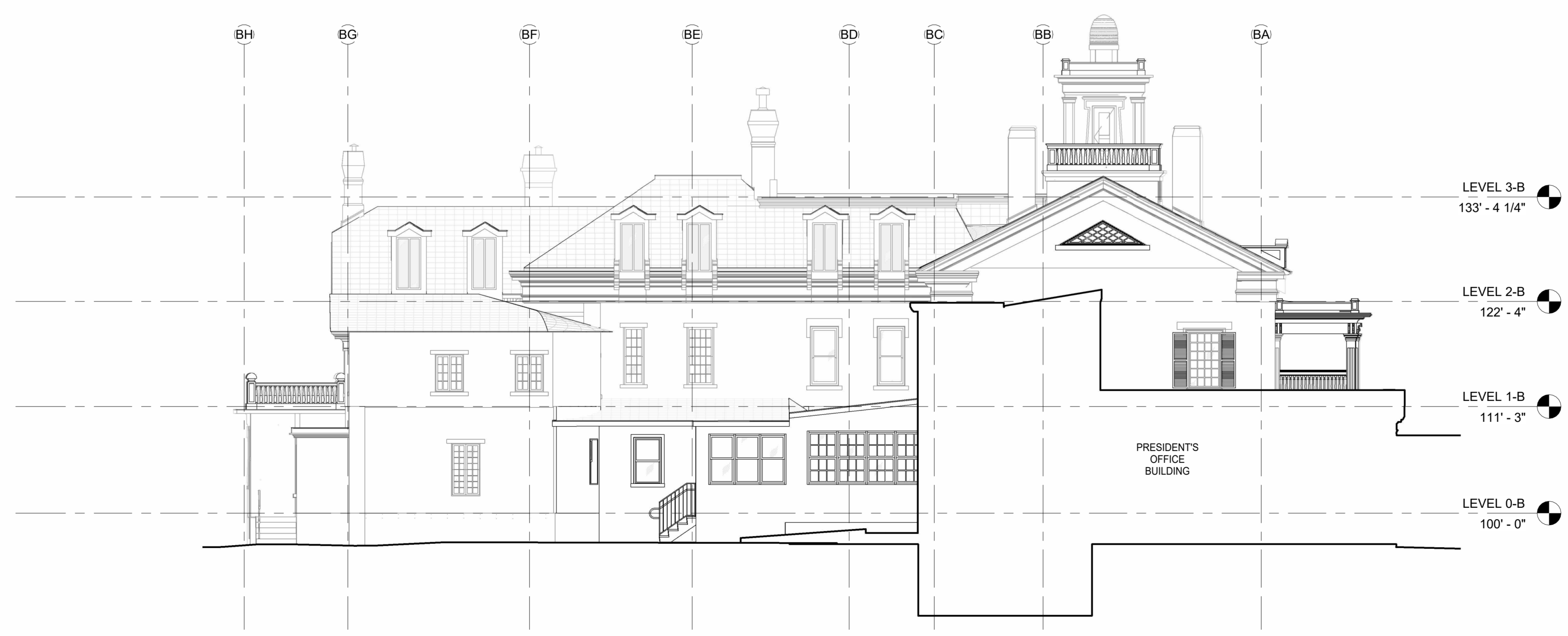
A1 WEST EXTERIOR ELEVATION - BEEHIVE HOUSE SCALE: 1/8" = 1'-0"
