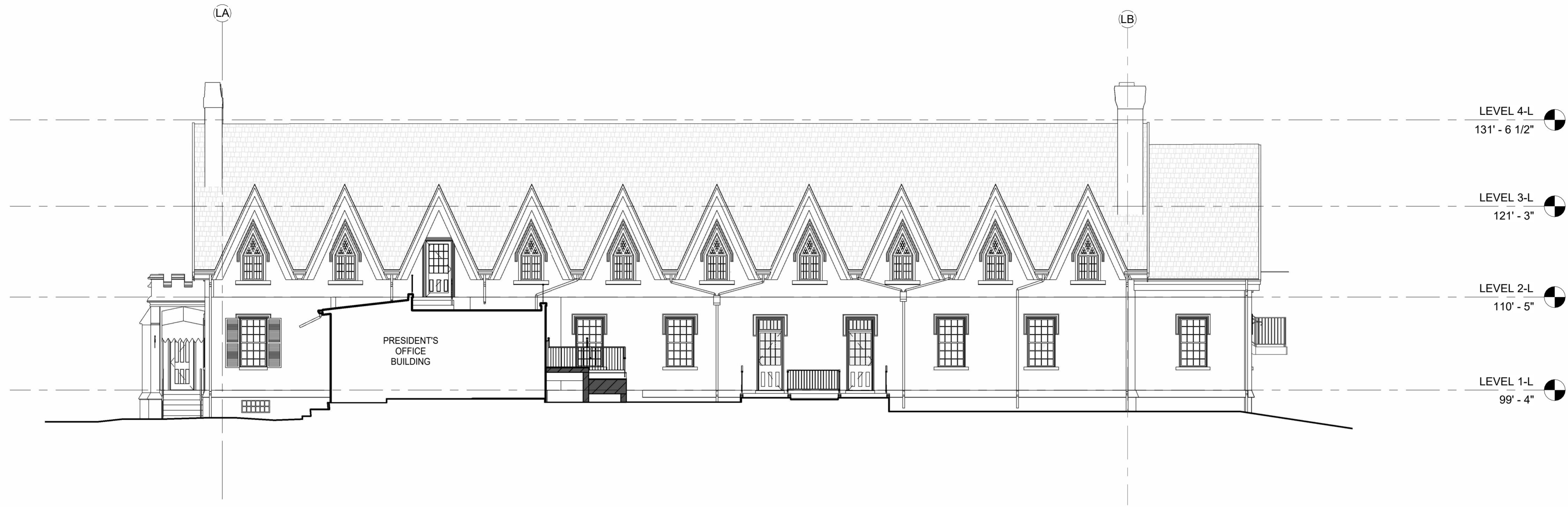
C1 EAST EXTERIOR ELEVATION - LION HOUSE SCALE: 1/8" = 1'-0"
