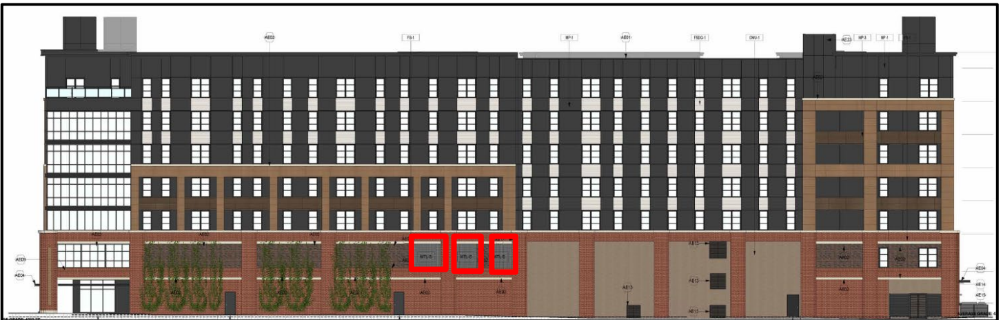
New parking ventilation locations
