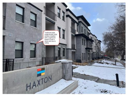
Another good example of appropriate windows installed with a reveal in a variety of façade materials.
