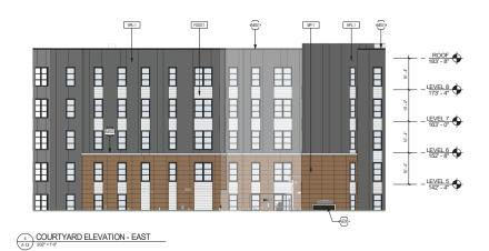
ARCHITECTURAL KEYNOTES AE01 PREFINISHED METAL COPING AE02 CAST STONE COPING AE05 INTAKE PENTHOUSE, REF. MECHANICAL AE07 ALUMINUM GLASS RAILING
