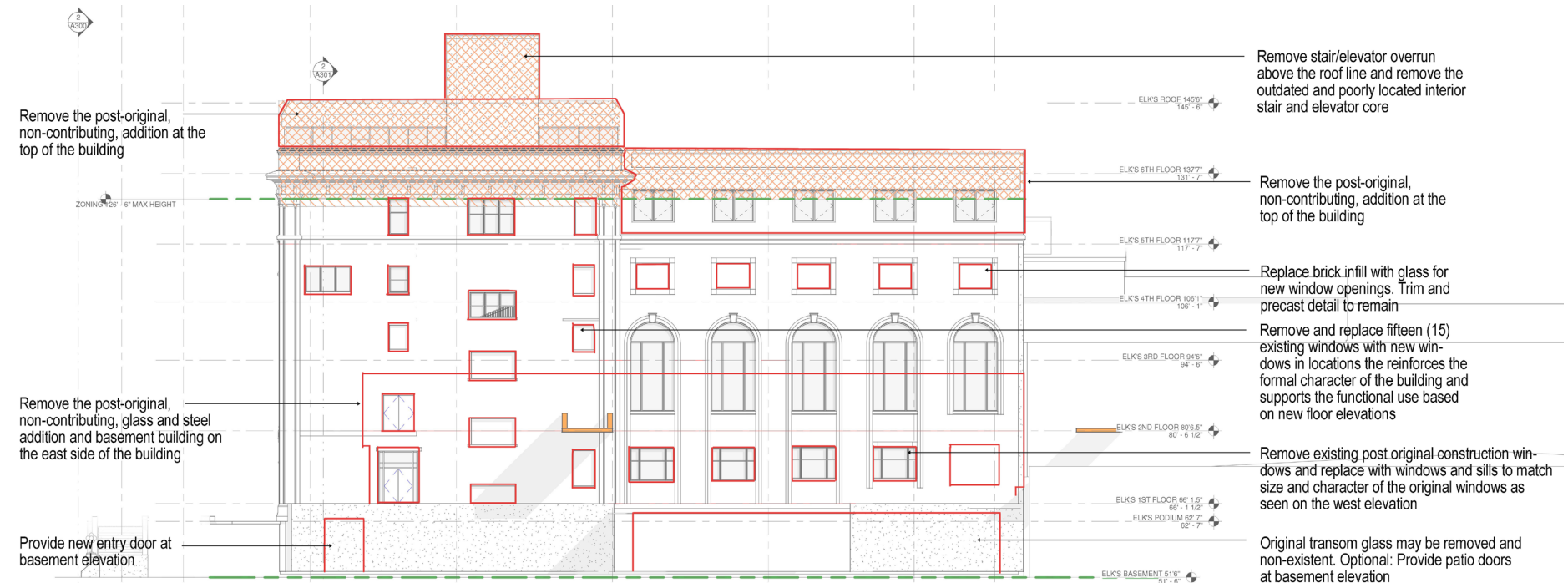
Elks Building - Proposed Alterations to Existing Building
