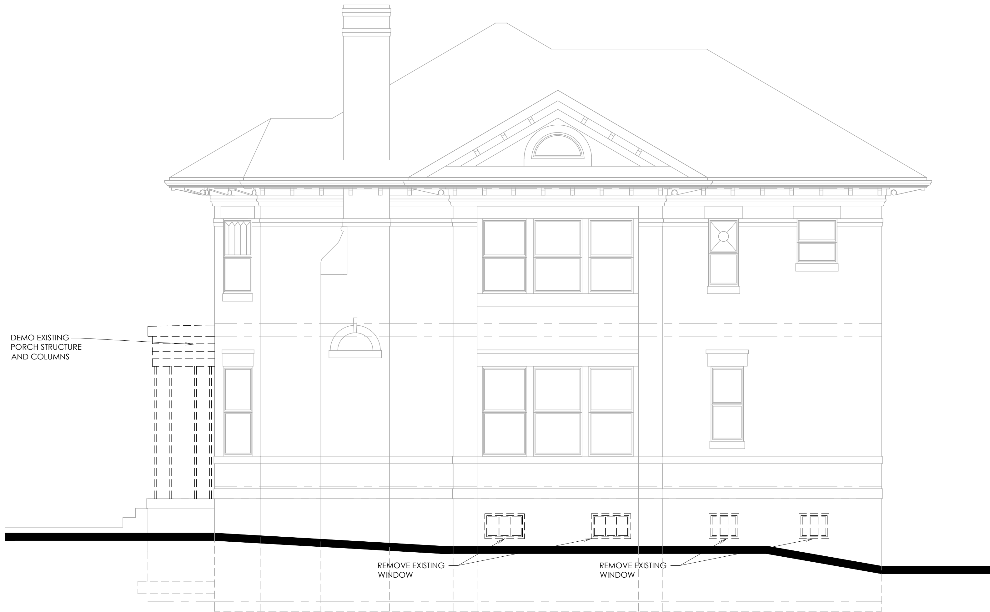
2 A3.2 EXISTING WEST ELEVATION SCALE (24x36): 1/4"=1'-0"
