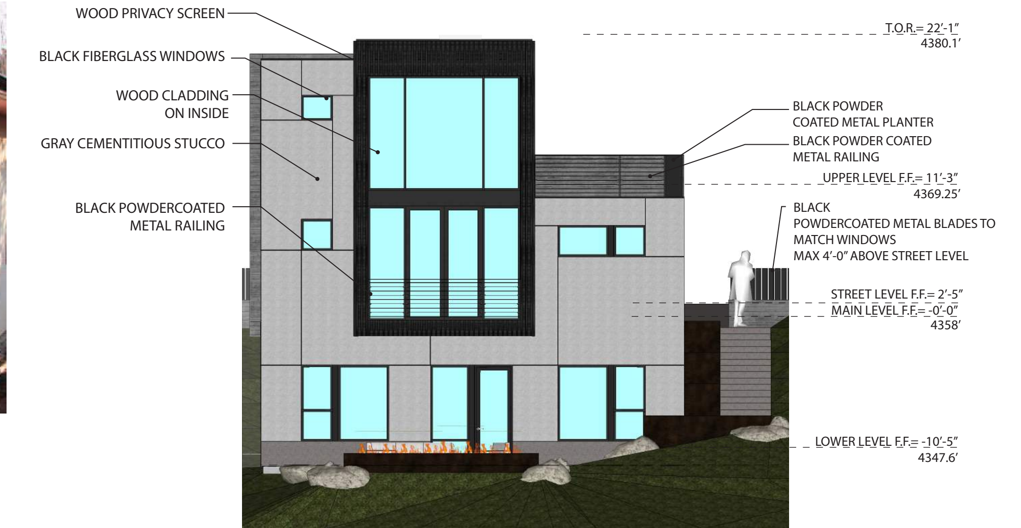
WEST ELEVATION - BACKSIDE OF PROPERTY SCALE: 1/4" = 1'-0"
