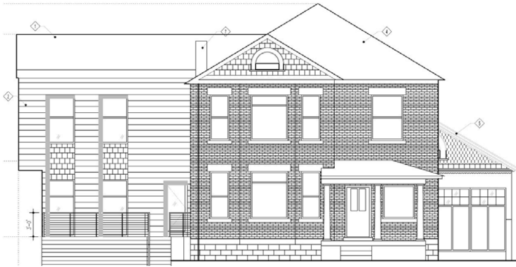
Front (east) elevation of historic home and proposed addition
