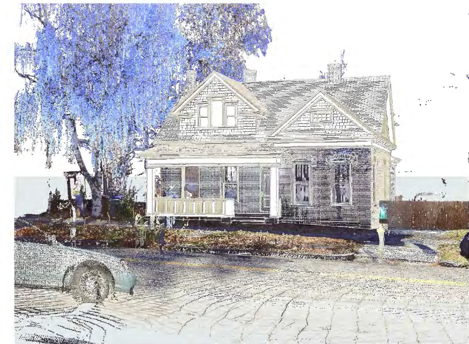
MODEL OF PROPOSED HISTORIC RENOVATION SUPERIMPOSED OVER POINT CLOUD SCAN DATA
