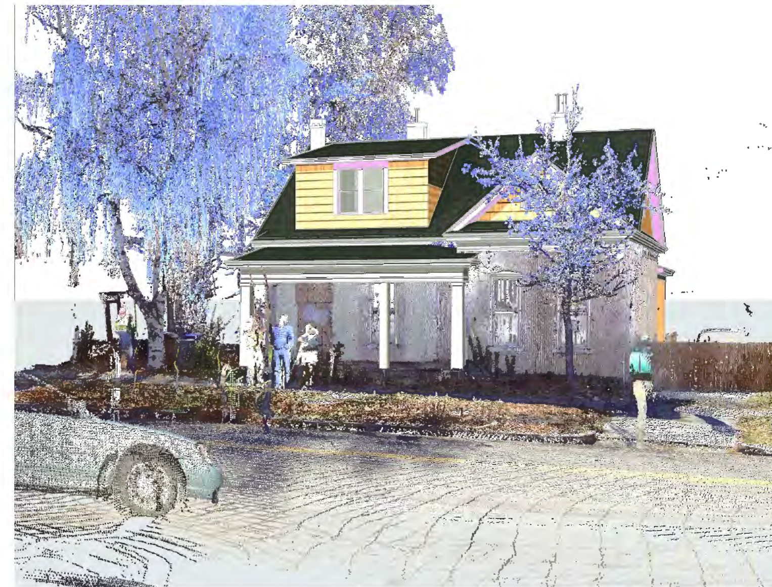
MODEL OF ORIGINAL HOUSE PRIOR TO 2017 EVENT SUPERIMPOSED OVER POINT CLOUD SCAN DATA
