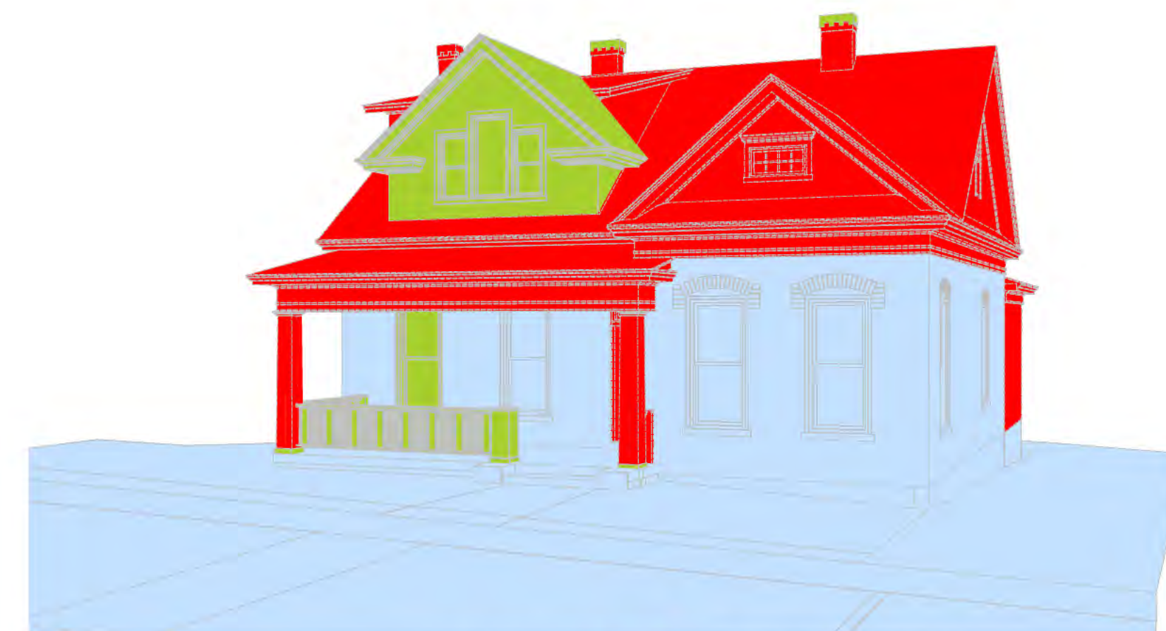
MODEL VIEW OF: ■ EXISTING ELEMENTS TO BE RECONSTRUCTED ■ ORIGINAL ELEMENTS ■ NEW ELEMENTS TO BE BUILT
