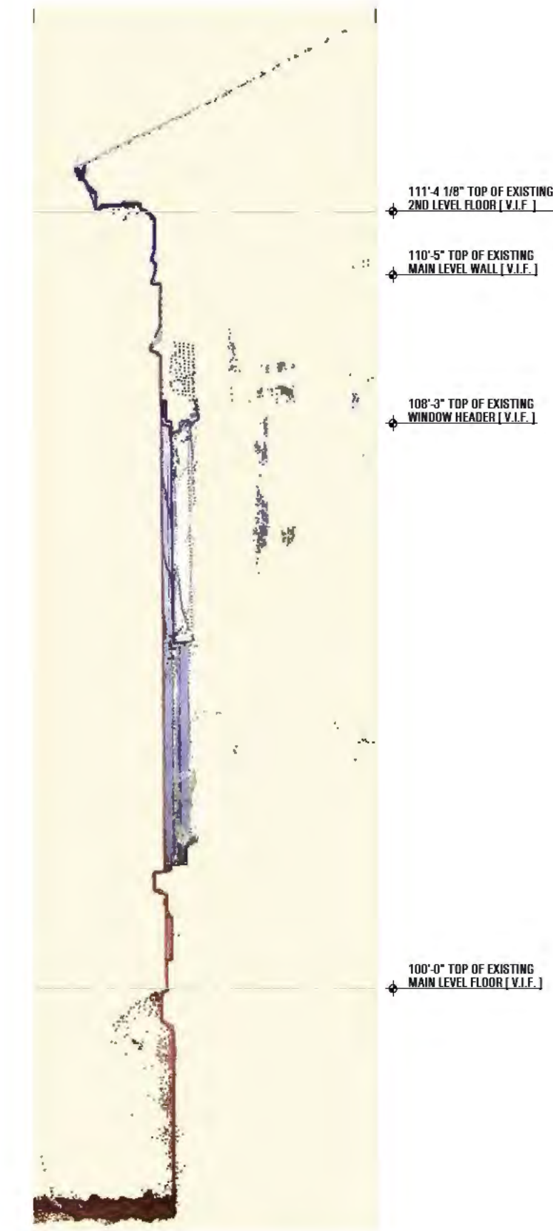
POINT CLOUD DATA - EAST BAY WALL SECTION 2B
