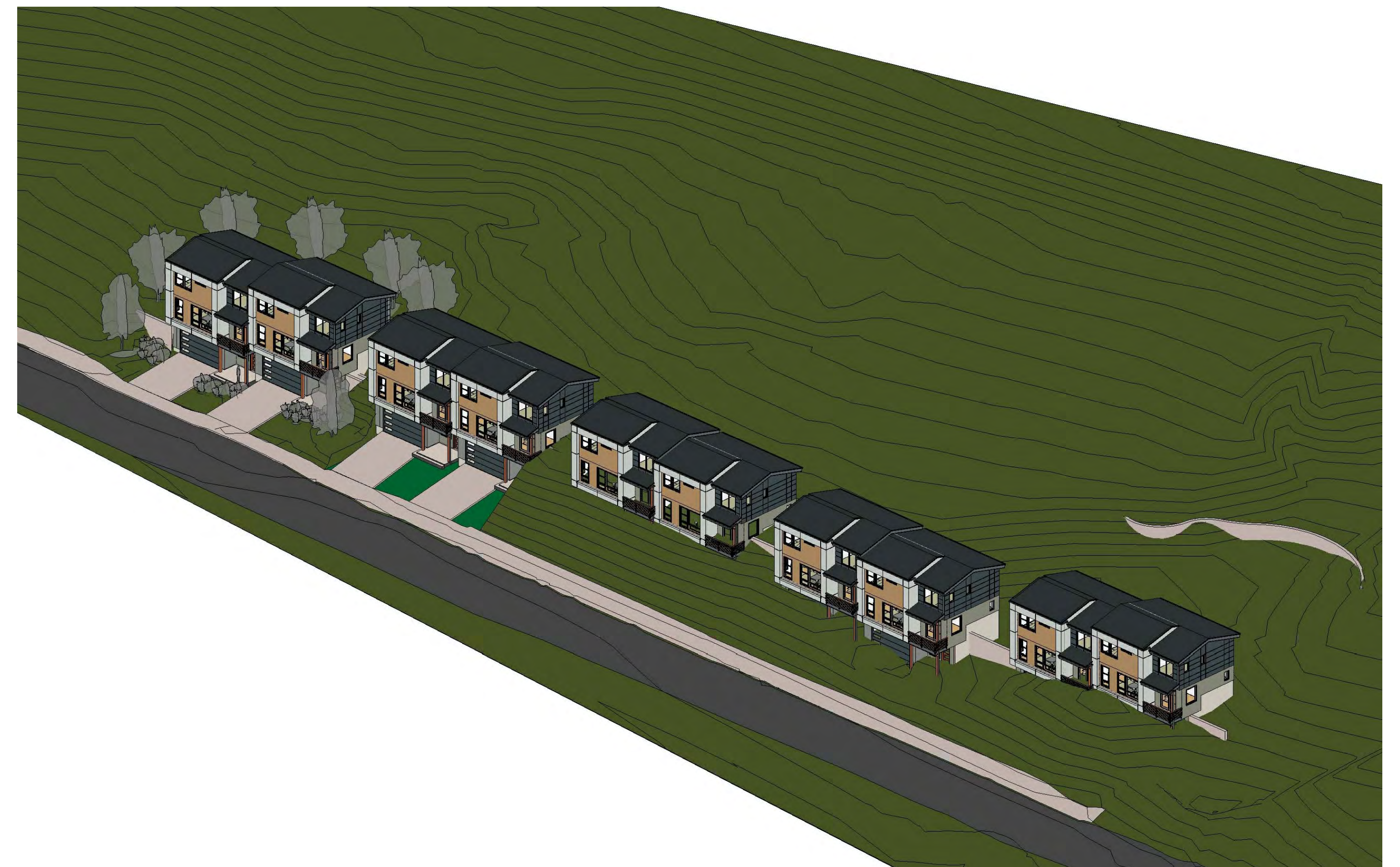
NORTH HOMES SHOWING EXCAVATION TO EXPOSE GARAGE LEVEL AND PROVIDE DRIVEWAY ACCESS TO STREET
