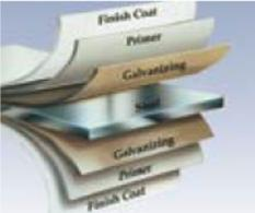
Steel skins are protected through a tough, layered coating system, including a hot-dipped galvanized layer, a protective metal oxide pretreatment and a baked-on primer and top coat.
