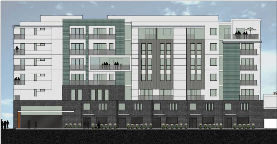
LEVEL ONE ELEVATION = 1,592 SF TOTAL AREA GLASS = 675 SF
