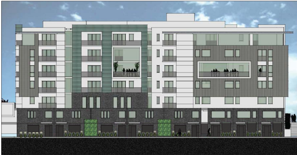
LEVEL ONE ELEVATION = 1,715 SF TOTAL AREA GLASS = 708 SF
