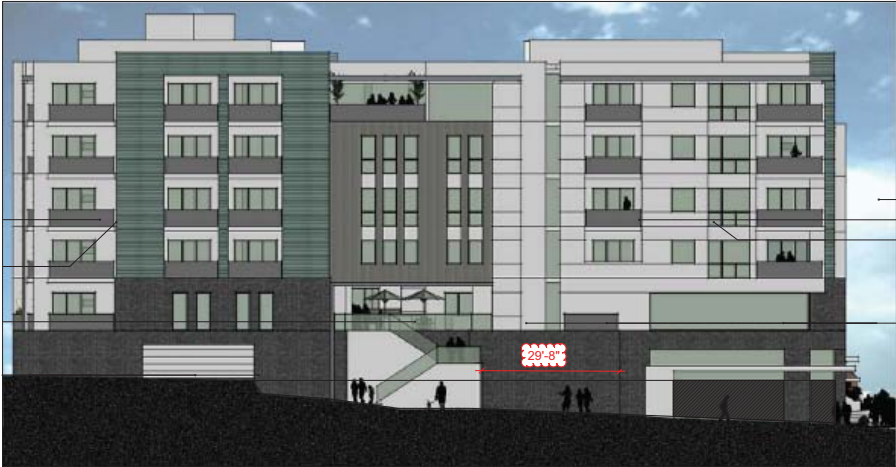
LEVEL ONE ELEVATION = 787 SF TOTAL AREA GLASS = 236 SF
