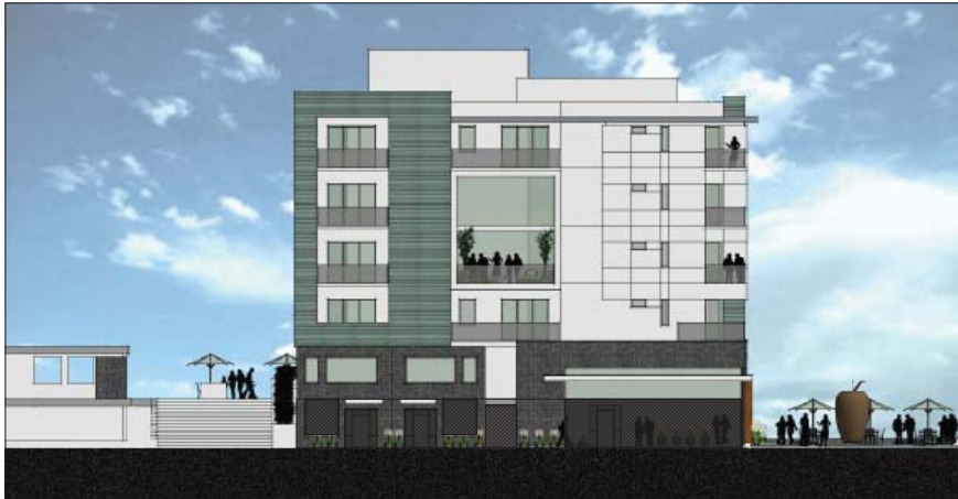
LEVEL ONE ELEVATION = 792 SF TOTAL AREA GLASS = 543 SF
