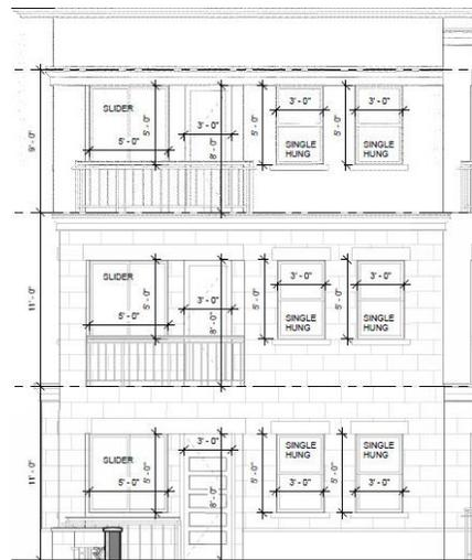
*Window detail west elevation*
