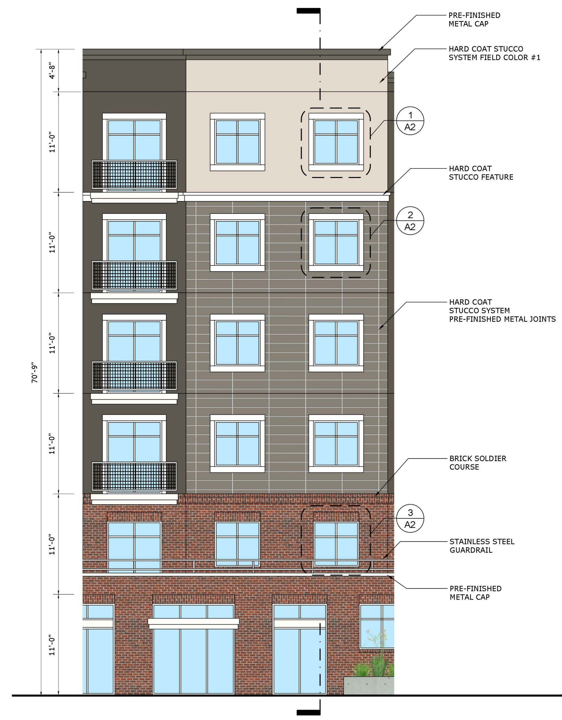
NORTH ELEVATION - WALL SECTION FINISHES AND WINDOW DETAILS
