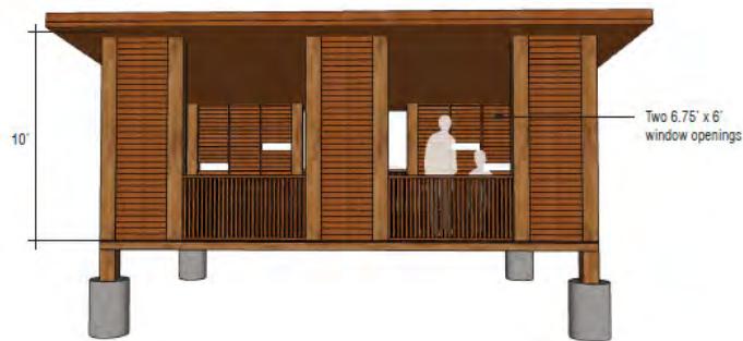
A "Duck Blind" Structure - Front View
