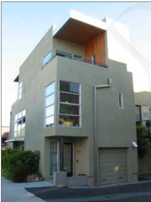
Graage access placed back from the street frontage and colored to blend with the facades,
