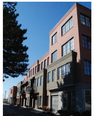
Designing a sense of transition in height, scale and character from principal to secondary street facades.
