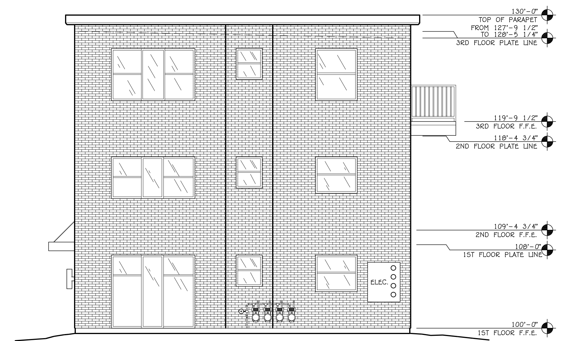
EAST ELEVATION - BUILDING A SCALE: 3/16" = 1'-0"
