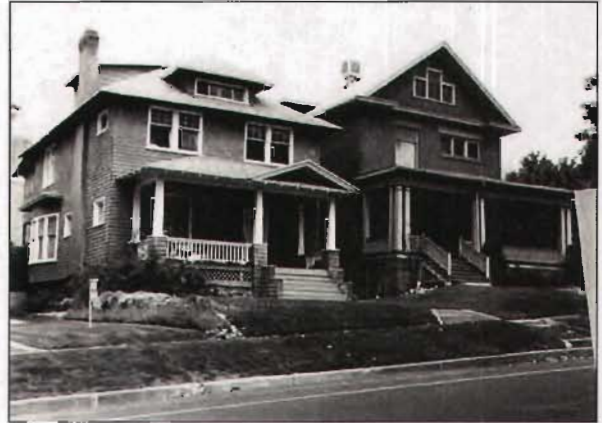
Because of its simplicity, the Foursquare lends itself to many styles. With thick square posts and exposed rafters it take on a Craftsman tone. With rounded porch columns and a pediment on the porch roof it becomes classical.
