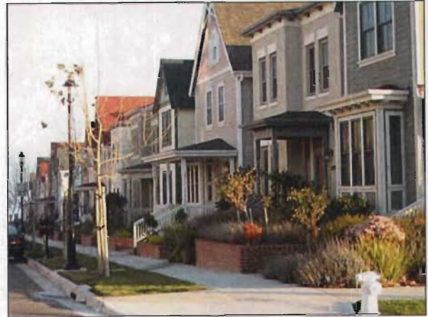
Several building designs and forms are used here to create variety and visual vitality, yet are designed to instill a strong vertical emphasis using facade or module width, reinforced by the rhythm established by single story porches and projecting window bays which share a common eaves height.
