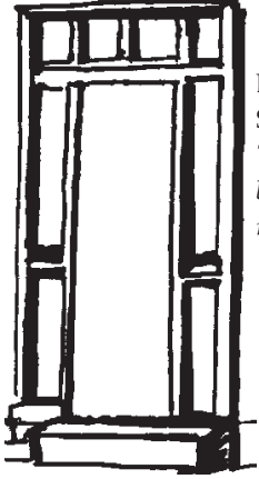
Doors with Transom and Sidelights Typically a wooden door flanked by sidelights and topped with a rectangular transom.
