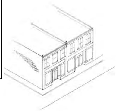
Most historic commercial buildings were designed with flat or sloping roofs.
