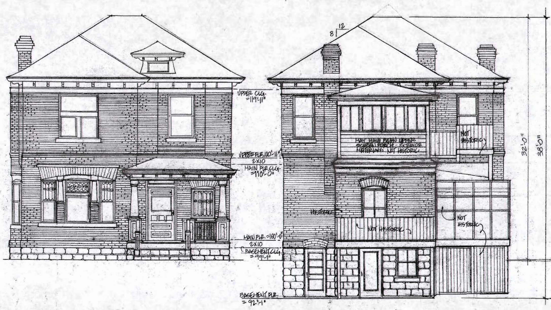
EXISTING NORTH ELEVATION 1/4" = 1'-0" NOTE: ALL MATERIALS PAINTED EXCEPT FRONT EXTERIOR DOOR.
